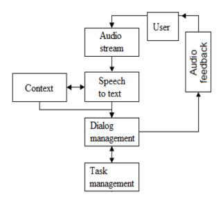
Fig. 1. An overview of the system architecture
