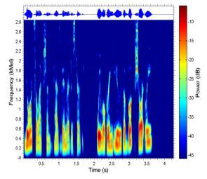
Fig. 4. The voice produced by the proposed system corresponding to the response text message "Your selection has been registered; we will bring you the book shortly". The produced voice waveform (top panel) and spectrogram analysis of the produced waveform (bottom panel).
