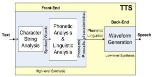
Fig. 2. Block diagram of a generic TTS system
